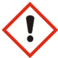
Acutely toxic(harmful), Irritant to skin, eyes or respiratory tract, Skin sensitizer, Hazardous to the Ozone layer.
